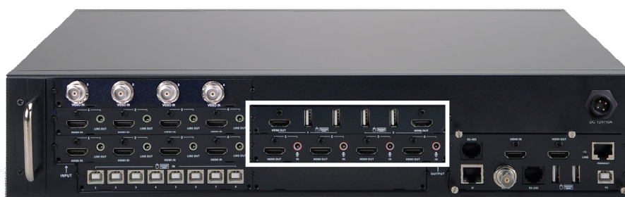
Figure 6-2 MS-2 Rear Panel: Multi-monitor Workstation Setup Example 1
