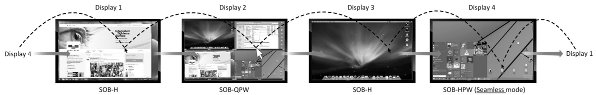
Figure 6-30 Multi-monitor Workstation with One Quad and Three Full Screen Displays: White cursor represents the Host cursor; dark cursor represents the cursor of the operating system
